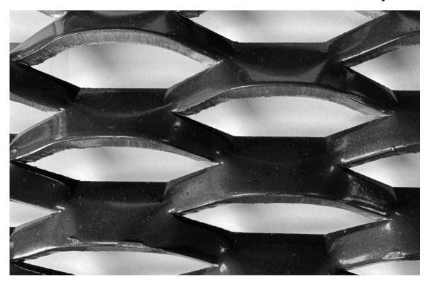
LW Pitch:121.92mmStrand Width:13.06mmSW Pitch:38.10mmThickness:6.00mmWeight:32.22 kg / m2Open Area:31%
